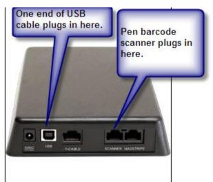
Once this is plugged into the computer follow the steps below. Remember the user may have to hold the pen at various angles to it to read the barcode.
